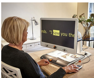
Control knobs for video magnifier
