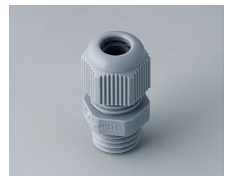
C2312418 Cable gland M12x1.5 PA 6 silver grey RAL 7001 IP 68 opt.
