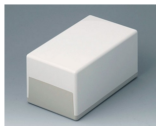
A9041065 FLAT-PACK CASE 189 H, Vers. I ABS (UL 94 HB) off-white RAL 9002 189x110x97mm IP 40
