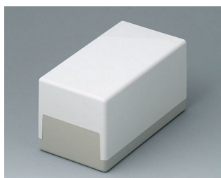
A9021065 FLAT-PACK CASE 120 H, Vers. I ABS (UL 94 HB) off-white RAL 9002 120x65x65mm IP 40
