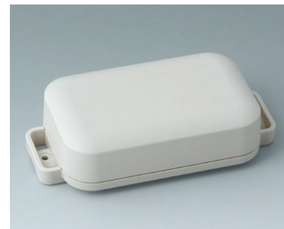
C3206207 EASYTEC 100 ASA+PC (UL 94 V-0) off-white RAL 9002 121x62x31mm IP 65 opt., IP 40
