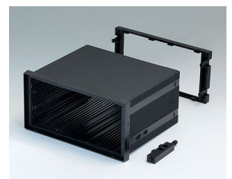
B6043041 DIN-MODULAR CASE TYPE A PPO (UL 94 V-0) black RAL 9005 144x72x109mm
