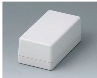
A9404341 SHELL-TYPE CASES G 85, Vers. I ABS (UL 94 HB) off-white RAL 9002 45x85x33mm IP 65 opt.
