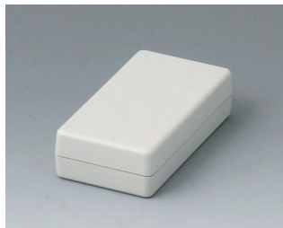
A9404331 SHELL-TYPE CASES G 85, Vers. I ABS (UL 94 HB) off-white RAL 9002 45x85x22mm IP 65 opt.
