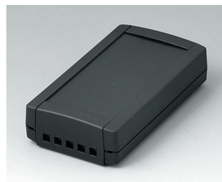
B1055469 TOPTEC 123 F, Vers. II ABS (UL 94 HB) black RAL 9005 123x68x30mm IP 40
