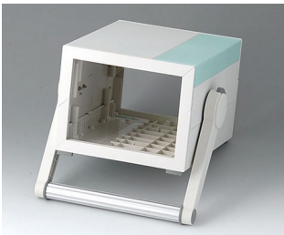
B2213315 MEDITEC E 160, with handle bar ABS (UL 94 HB) off-white RAL 9002 160x200x124mm IP 40
