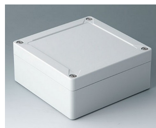
C7013031 IN-BOX ABS (UL 94 HB) light grey RAL 7035 124x122x55mm IP 66, IP 67, IK 08
