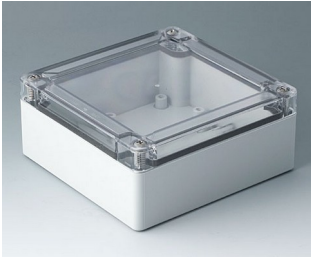
C7013034 IN-BOX ABS/PC (UL 94 HB) light grey RAL 7035 124x122x55mm IP 66, IP 67, IK 07
