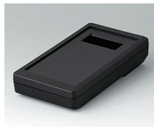
A9073219 DATEC-MOBIL-BOX S, Vers. II ABS (UL 94 HB) black RAL 9005 152x83x33.5mm IP 65 opt.
