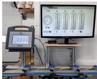
Monitoring system for cleaning nozzles
