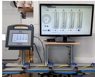
Monitoring system for cleaning nozzles
