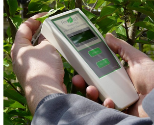
Chlorophyll fluorimeter for plant screening
