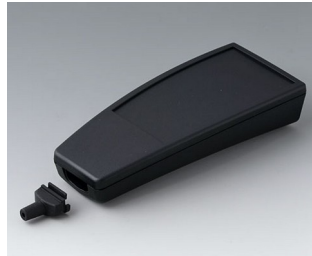
A9068339 SMART-CASE XL, Vers. IV ABS (UL 94 HB) black RAL 9005 168x74.4x35.4mm IP 65 opt., IP 40
