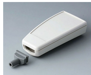
A9066127 SMART-CASE M, Vers. III ABS (UL 94 HB) off-white RAL 9002 96x47x24mm IP 40
