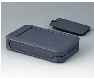
A9052118 SOFT-CASE L ABS (UL 94 HB) lava 73x117x24mm IP 40
