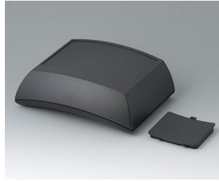
B7025109 ERGO-CASE L, high ABS (UL 94 HB) black RAL 9005 150x200x69mm IP 54 opt.
