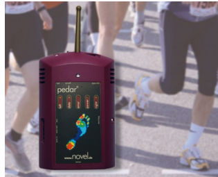
Dynamic pressure measuring between foot and shoe
