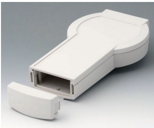
A9079107 DATEC-CONTROL L, Vers. I ABS (UL 94 HB) off-white RAL 9002 266x144x60mm IP 54 opt.
