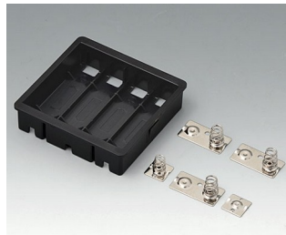
EZ050609 Battery compartment, 4 x AA ASA+PC (UL 94 V-0) black RAL 9005
