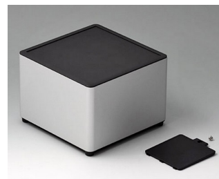
ES149059 SYNERGY S140 Aluminium AIMgSi 0.5 matt anodised 140x140x100mm IP 40
