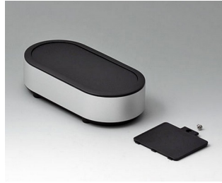
EO163059 SYNERGY O160 Aluminium AIMgSi 0.5 matt anodised 160x80x40mm IP 40
