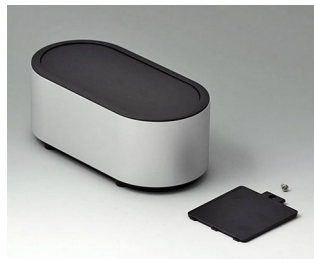
EO186059 SYNERGY O180 Aluminium AIMgSi 0.5 matt anodised 180x90x70mm IP 40
