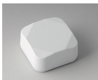
B1802217 MINI-DATA-BOX S40, high ASA+PC (UL 94 V-0) traffic white RAL 9016 40x40x20mm IP 65 opt., IP 40
