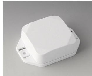
B1804227 MINI-DATA-BOX SF50, high, with flanges ASA+PC (UL 94 V-0) traffic white RAL 9016 50x50x20mm IP 65 opt., IP 40
