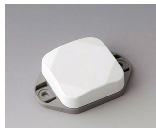
B1802126 MINI-DATA-BOX SF40, flat, with flanges ASA+PC (UL 94 V-0) traffic white RAL 9016 40x40x15mm IP 65 opt., IP 40
