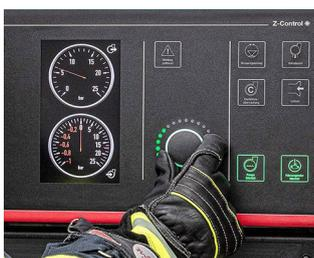
Control element for pump control station
