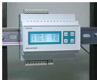
Power measuring device for energy analysis
