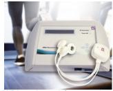
WBA receiver unit for measuring biosignals
