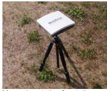
Measuring station for stationary field measurements
