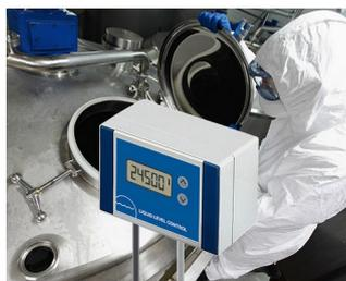
Fill level measurement in process technology
