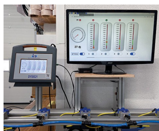
Monitoring system for cleaning nozzles
