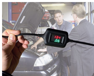
Voltage and current display during trickle charging
