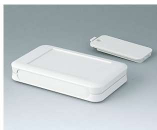
A9051117 SOFT-CASE M ABC (UL 94 HB) белый RAL 9002 65x105x19mm IP 40
