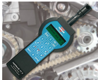
Pretension tester for V-belts and toothed belts
