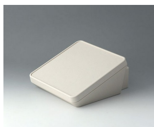
B4418307 PROTEC 180, Vers. III ASA+PC (UL 94 V-0) off-white RAL 9002 180x201x92mm IP 65 opt.
