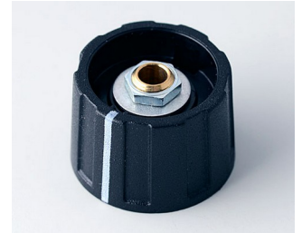
A2623040 ROUND KNOB 23, with line ABS (UL 94 HB) black RAL 9005 23x15mm 4mm
