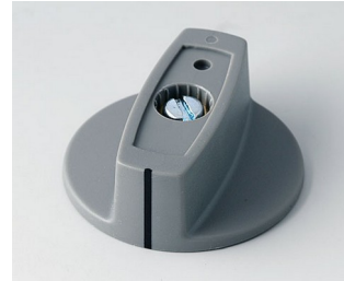
A2440068 SPINDLE-SHAPED KNOB 40, with line ABS (UL 94 HB) dusty grey RAL 7037 40x16mm 6mm
