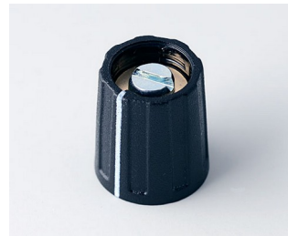
A2613060 ROUND KNOB 13.5, with line ABS (UL 94 HB) black RAL 9005 13x15mm 6mm
