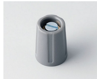
A2510048 ROUND KNOB 10, without line ABS (UL 94 HB) dusty grey RAL 7037 10x14mm 4mm
