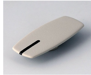
A5031107 Cover 31, with line ABS (UL 94 HB) pebble grey RAL 7032
