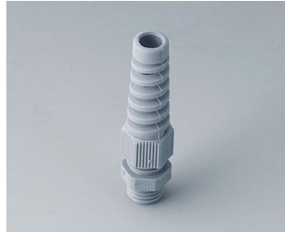
C2312518 Cable gland M12x1.5, bending protection PA 6 silver grey RAL 7001 IP 68
