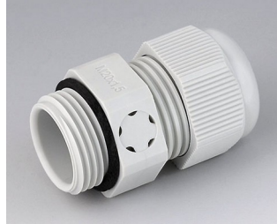
C2320917 Cable gland M20x1.5, pressure compensation PA 6 (UL 94 V-0) light grey RAL 7035 IP 68
