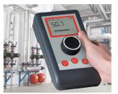
Find compressed air leaks using ultrasound
