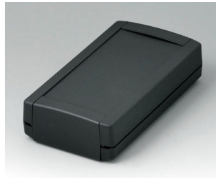
B1065369 TOPTEC 154 F, Vers. I ABS (UL 94 HB) black RAL 9005 154x84x38mm IP 40
