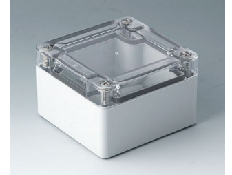
C7008015 IN-BOX PC light grey RAL 7035 84x82x55mm IP 66, IP 67, IK 08
