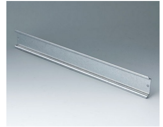
C7118077 Standard DIN rail, Type TH 35 Steel 283,5x35x7,5mm
