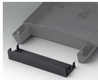
B3322918 Infill cover 220 ASA+PC (UL 94 V-0) lava
