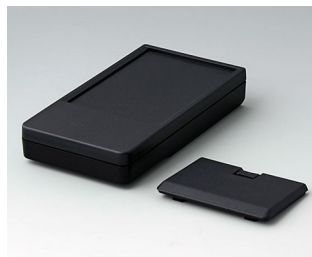
A9072129 DATEC-POCKET-BOX L ABS (UL 94 HB) black RAL 9005 120x65x22mm IP 41
