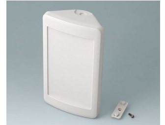
B4610207 SMART-CONTROL M, Vers. II ASA+PC (UL 94 V-0) off-white RAL 9002 173x101x59mm IP 55 opt., IP 40
