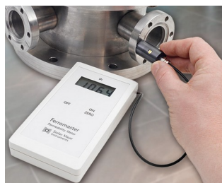
Ferromaster Permeability Meter
