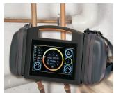
Mobile radio remote control unit for orbital welding system
