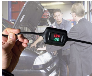
Voltage and current display during trickle charging
