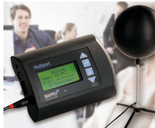
Multipoint with integrated datalogger
