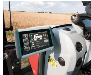
ISOBUS terminal for tractors and self-propelled machines
