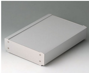
B3407033 SMART-TERMINAL 240 Aluminium AlMgSi 0,5 matt anodised 244x170x50mm
