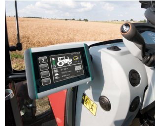
ISOBUS terminal for tractors and self-propelled machines
