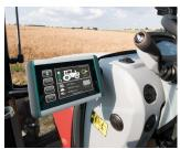
ISOBUS terminal for tractors and self-propelled machines
