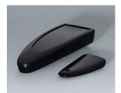
B2803016 STYLE-CASE M PMMA (IR) (UL 94 HB) black RAL 9005 147x56x27mm IP 65 opt., IP 40
