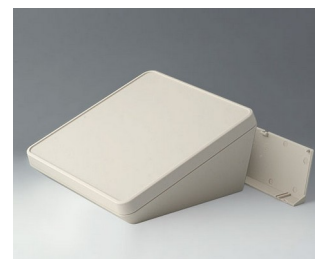
B4422207 PROTEC 220, Vers. II ASA+PC (UL 94 V-0) off-white RAL 9002 220x220x108mm IP 65 opt.
