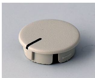
A4116107 Cover 16, with line ABS (UL 94 HB) pebble grey RAL 7032
