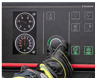
Control element for pump control station
