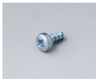
A0306031 Self-tapping screws 3 x 6 mm (PZ1)
