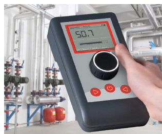
Find compressed air leaks using ultrasound
