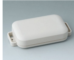
C3206107 EASYTEC 100 ASA+PC (UL 94 V-0) off-white RAL 9002 121x62x26mm IP 65 opt., IP 40
