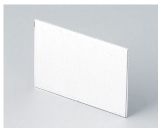
B6112112 Rear panel Aluminium matt anodised 42,2x29,6x1mm
