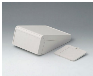
B4054317 UNITEC S, 1.4/1.4 ABS (UL 94 HB) off-white RAL 9002 125x177x69mm IP 40
