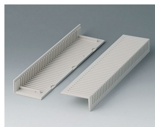
B2021007 Side trims 220, with ventilation ABS (UL 94 HB) off-white RAL 9002
