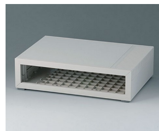
B2211007 MEDITEC D 160, without handle bar ABS (UL 94 HB) off-white RAL 9002 290x200x74mm IP 40
